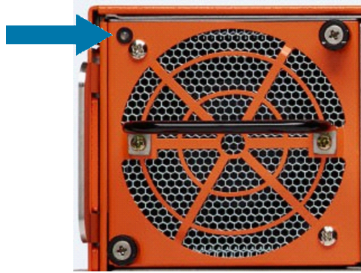
Figure 6 Individual Fan LED Location on GigaVUE-HC3 Rear
